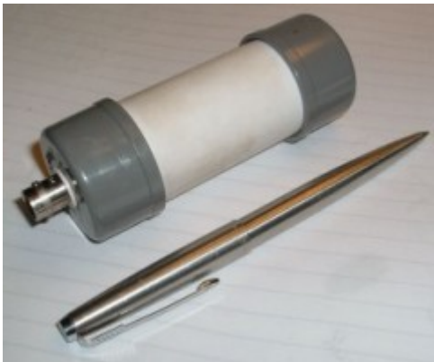
Fig. 5 De mini-whip in (witte) PVC-pijp
